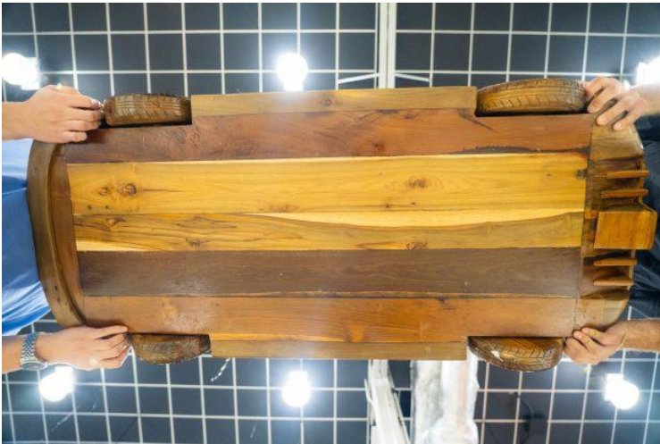
The underside is flat with an upturned rear diffuser area and conceals the two steel axles. The model measures approximately 48.5" long, 24" wide, and 13" tall.
